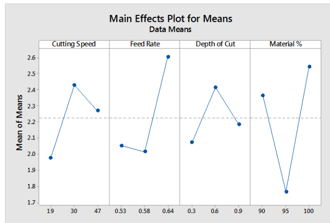
Fig.8. Main effects for means
